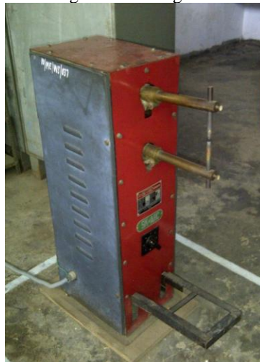
Fig3 Picture of spot welding machine used for experiment
