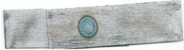
Fig4. Picture of welded specimen
