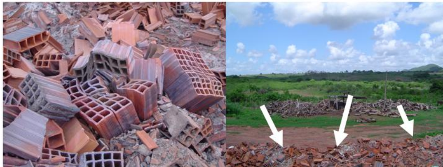
Fig. 4 Fire solid residues (left) and disposal of residues (right).
