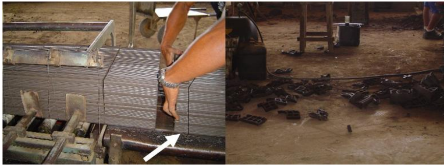
Fig. 3 Uneven cutting of the pieces (left), generating solid residues (right).
