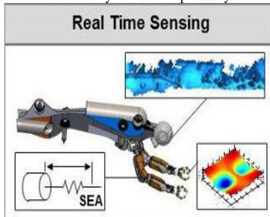
Haptic-enabled humanoid robot for underwater exploration uses hybrid actuation. (Courtesy of Stanford University)
