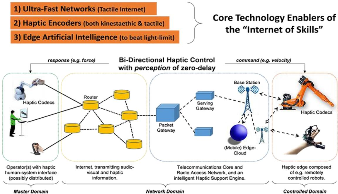
Fig. 2 High level architecture of the Internet of Skills and required building blocks.
