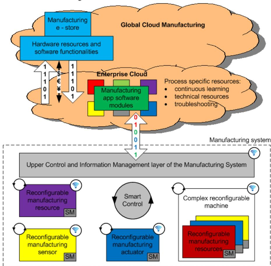
Fig. 3. Simplified view of the proposed IoT architecture for Manufacturing
