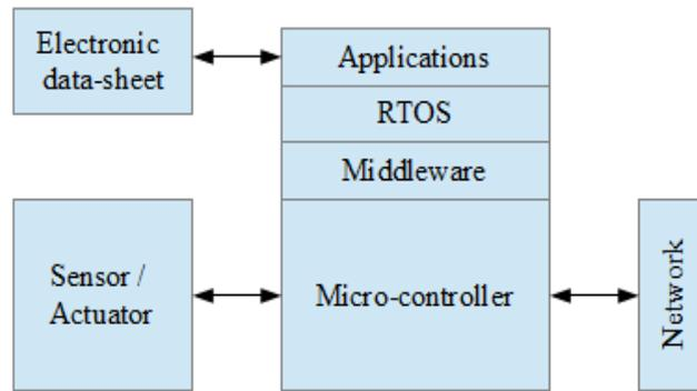
Fig. 4. Smart manufacturing resource architecture for IoT
