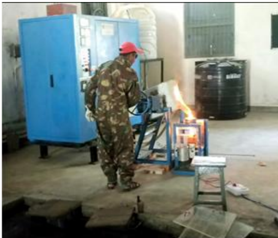
Fig.2. Pouring of Molten Copper
