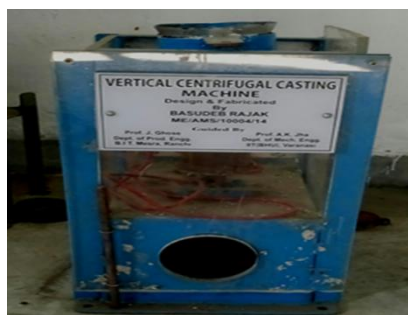
Fig.1. Experimental setup of Vertical centrifugal casting.
