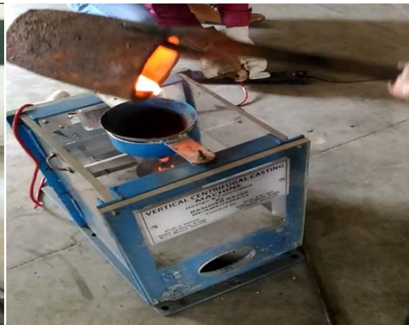
Fig.3. Pouring of molten Aluminum
