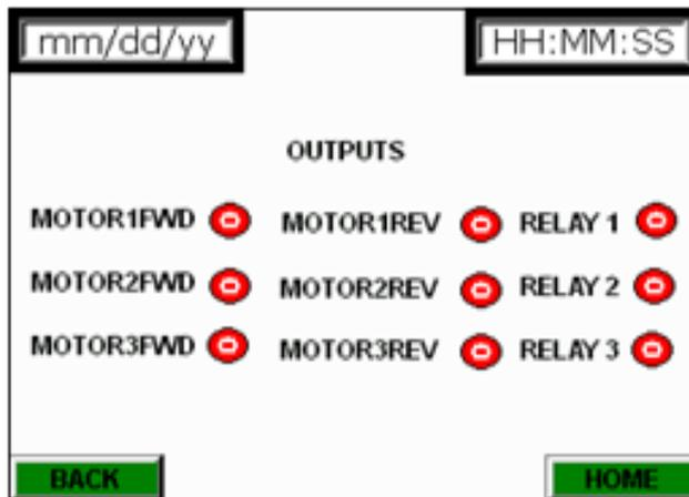
Figure 8 Working status of outputs in PLC by using HMI
