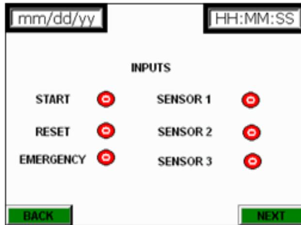
Figure 7 shows that working status of inputs in PLC by using HMI
