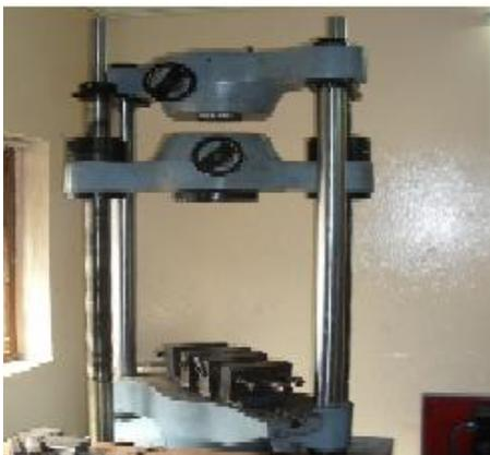
Figure.10. UTM for Flexural test
