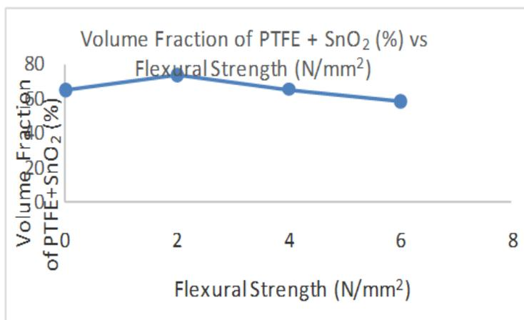
Figure 22 Volume Fraction of PTFE + SnO<sub>2</sub> (%) vs Flexural Strength (N/mm<sup>2</sup>)
