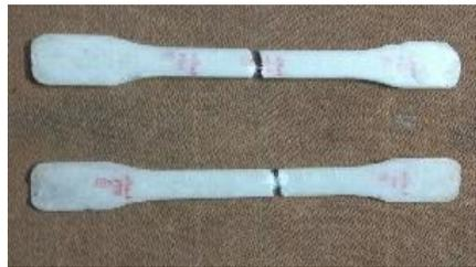
Figure 6. Sample with glass fiber + epoxy resin +  $\text{SnO}_2$  after tension test
