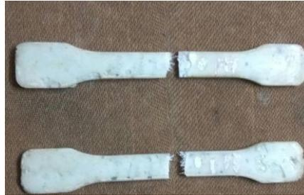
Fig 8. Sample with glass fiber + epoxy resin after tension test
