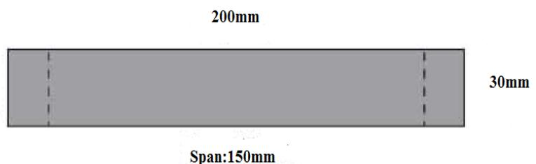
Figure. 11. Specimen dimension for flexural test
