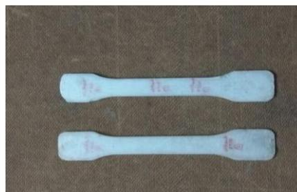
Figure 4. Sample with glass fiber + epoxy resin before tension test
