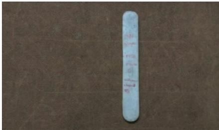
Figure 14. Sample with glass fiber + epoxy resin before flexural test
