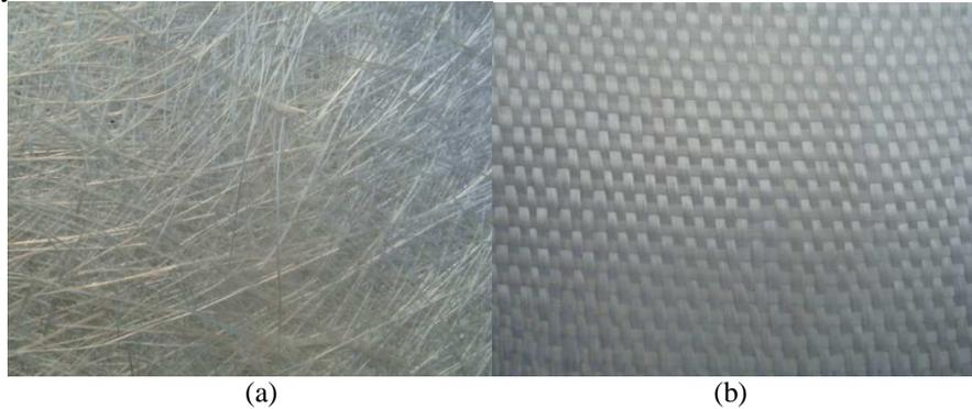
Figure. 1. E- Glass Fibers (a) CMS and (b) WRM
