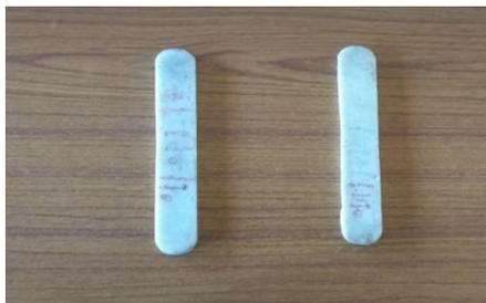
Figure 16. Sample with Fiber + epoxy resin + PTFE powder before flexural Test
