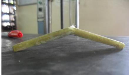
Figure 13. Specimen after flexural test
