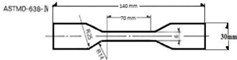
Figure 3. Tensile test specimen specifications as per ASTM D
