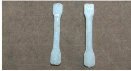
Fig 7. Sample with glass fiber + PTFE+ epoxy resin before tension test
