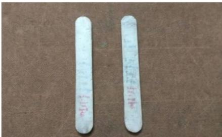
Figure 15. Sample with glass fiber + SnO<sub>2</sub> + epoxy resin before flexural test
