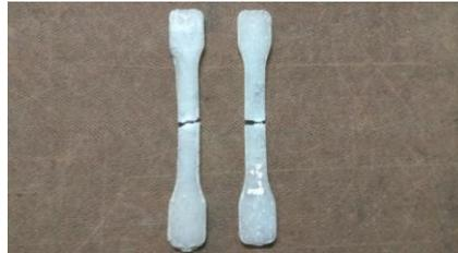
Figure 9. Sample with glass fiber + PTFE + epoxy resin after tension test
