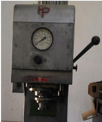
Fig.1. Hydraulic compacting machine
