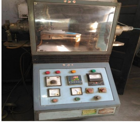
Fig.4. Electrical furnace set-up for conventional sintering
