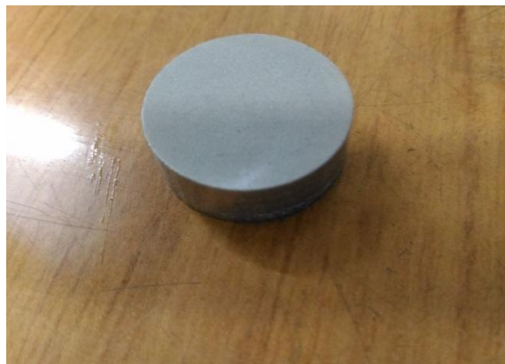
Fig.2. Specimen prepared after compaction
