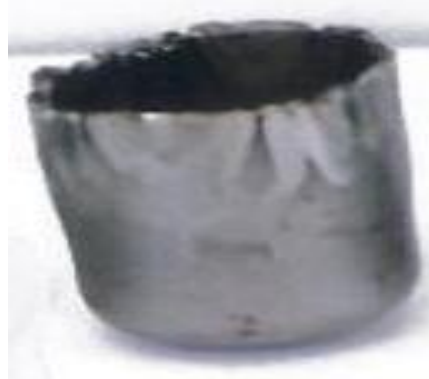
Fig. 3 Wrinkling in deep drawing
