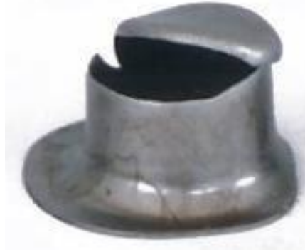
Fig. 2 Fracture in deep drawing [4]
