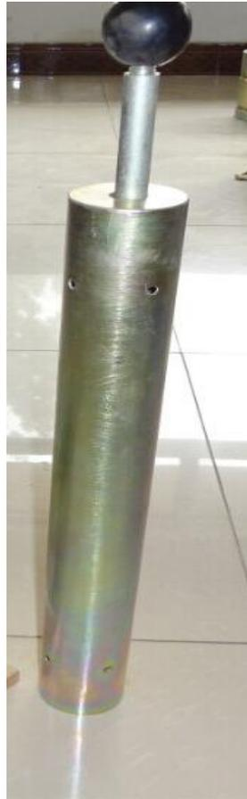
Fig. 4: Hammer of modified proctor.
