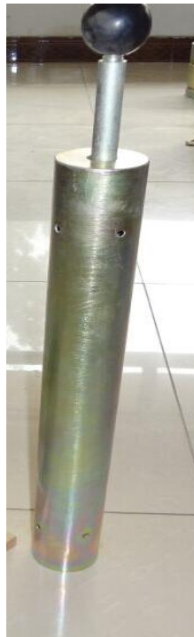
Fig. 4: Hammer of modified proctor.
