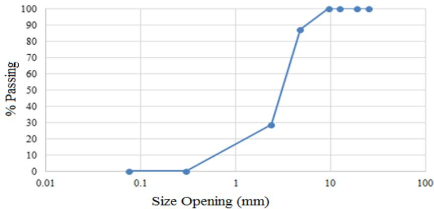
Fig. 1: Particle size distribution of plastic waste.
