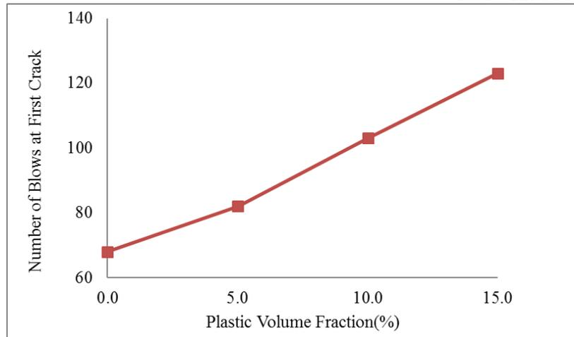
Fig. 7: First crack impact resistance against volume fraction of plastic.
