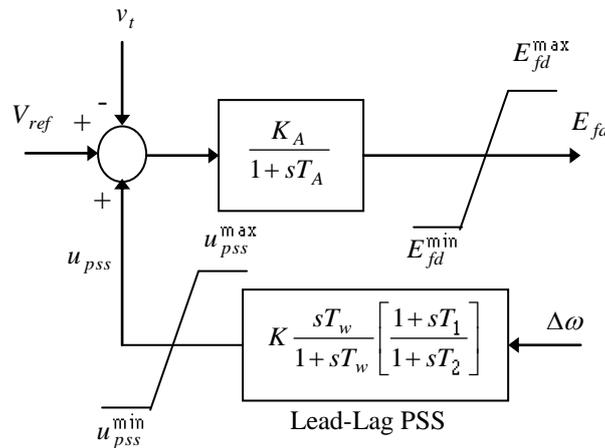
Fig. 3 IEEE Type-ST1 Excitation System with PSS
