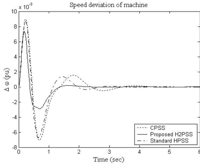
Fig. 5 Responses with 10% Step in  $V_{ref}$  for Case 2
