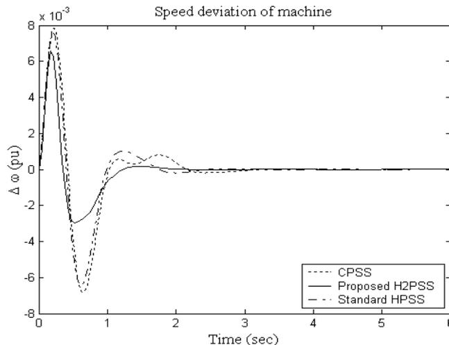
Fig. 4 Responses with 10% Step in  $V_{ref}$  for Case 1
