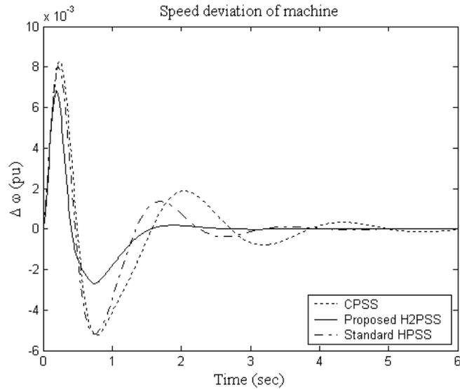
Fig. 8 Responses with Fault Disturbance for Case (a)
