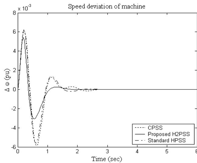
Fig. 7 Responses with 10% Step in  $V_{ref}$  for Case 4
