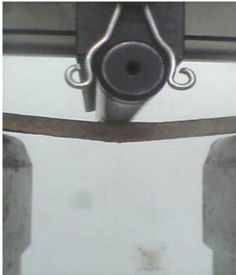
Fig.12 three point bending test in UTM
