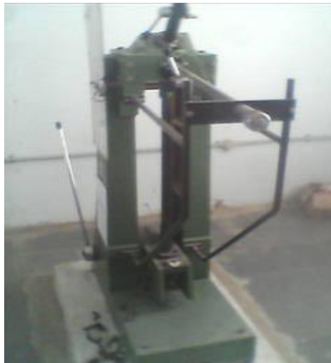
Fig.13 IZOD impact testing equipment
