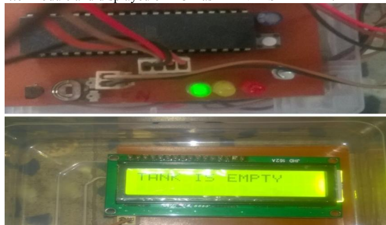
Fig. 5 Indication of LED and LCD when tank is empty
