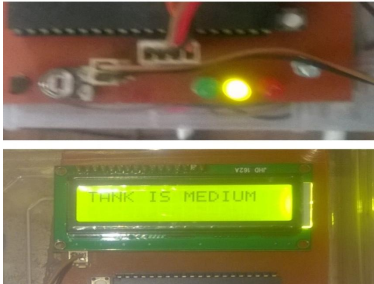
Fig. 6 Indication of LED and LCD when tank is medium
