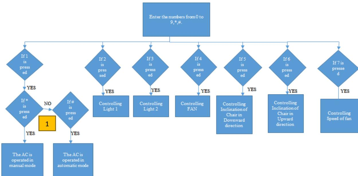
Fig 4: Flow chart of the keypad functions
