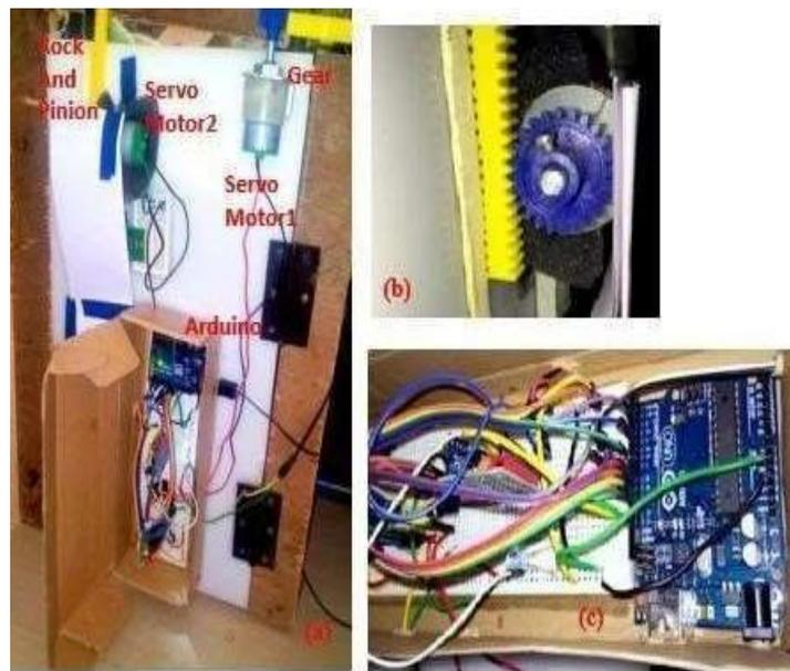
Fig 2: (a) Experimental circuit setup (b) Gear with rack and pinion at Motor 2 (c) Arduino connected to the circuit board DC electric motor which works by dividing a full rotation into number of equal steps.
