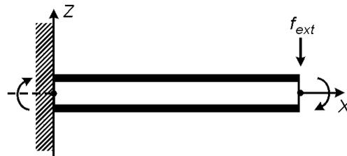
(b) A aluminum Timoshenko cantilever beam bonded with surface mounted piezoelectrics
