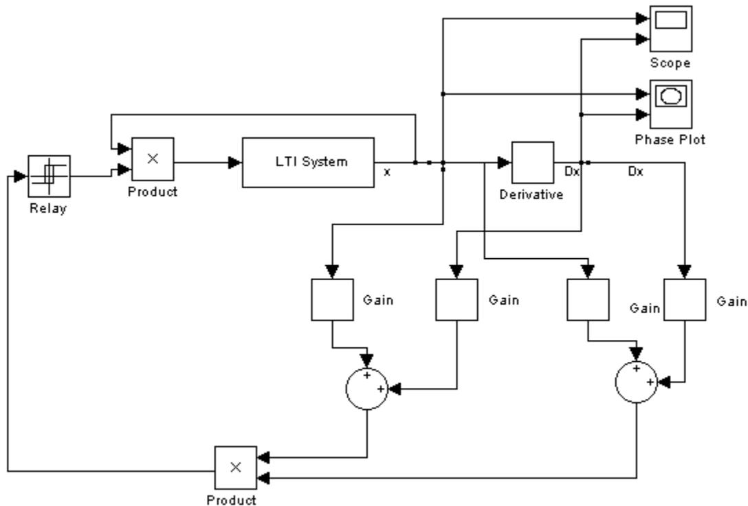
Fig. 2 : Control methodology used for vibration suppression by Simulink diagram
