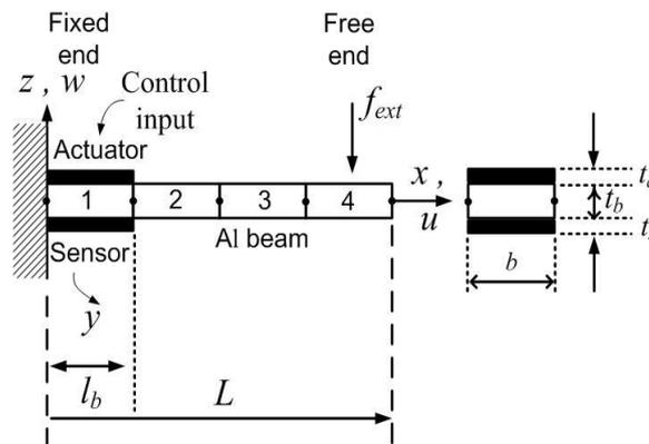
Fig. 2 : Model 1 (PZT placed at FE position 1, fixed end)
