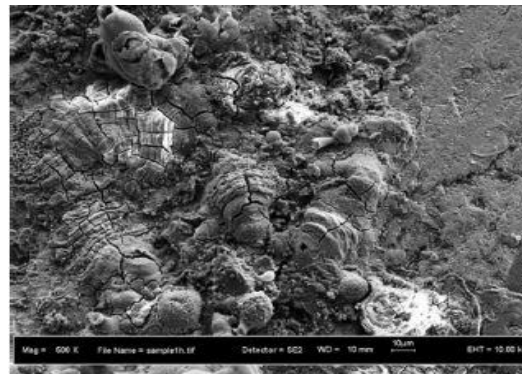
Fig. 2. FESEM of control steel specimen (no chloride)
