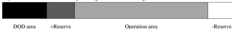
Fig. 2 Concept of storage allocation for optimized scheduling and handling generation and load uncertainties [15]
