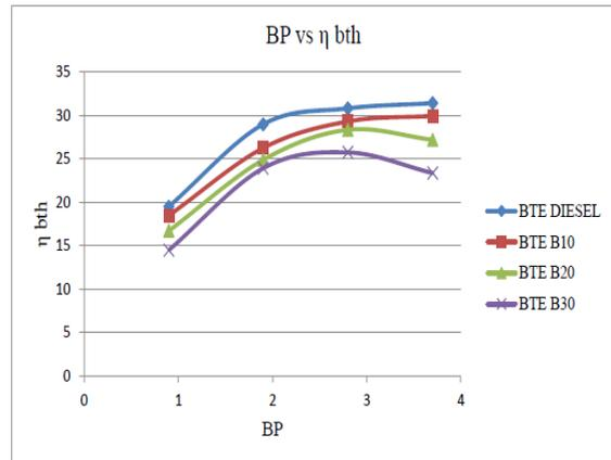
Figure 2: BP vs Break Thermal Efficiency for IP of 180 Bar
