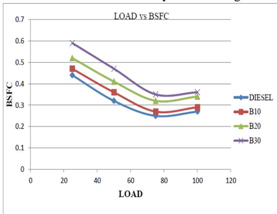
Figure 3: Load vs BSFC for IP of 180 Bar
