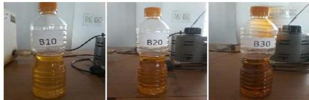
Figure 11: Different Blends of Biodiesel i.e. B-10, B-20 and B30.
