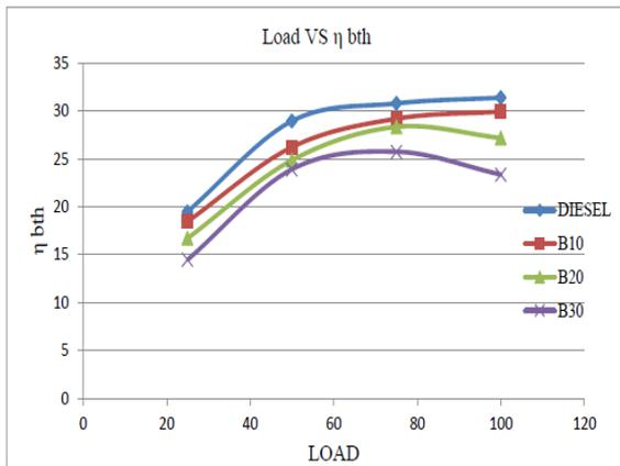
Figure 1: Load vs Break thermal efficiency for IP of 180 Bar
