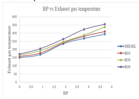
Figure 6: BP vs EGT foe IP of 180 Bar
