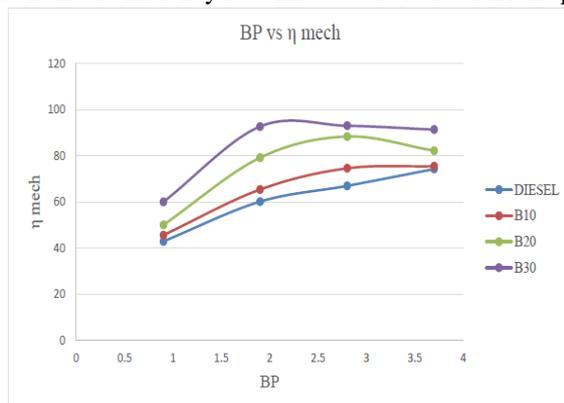
Figure 5: BP vs Mechanical Efficiency for IP of 180 Bar
