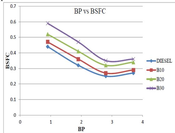
Figure 4: BP vs BSFC for IP of 180 Bar
