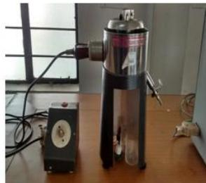
Figure 13: cleave land Open cup Flash and fire Point Apparatus      Figure 14: Red wood Viscometer Apparatus
