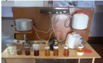
Figure 5: Transesterification Reactor set up
