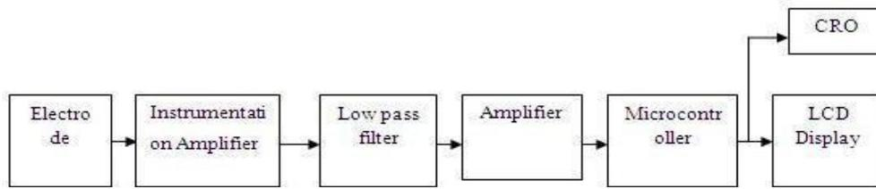
Figure 4. ECG generation unit
