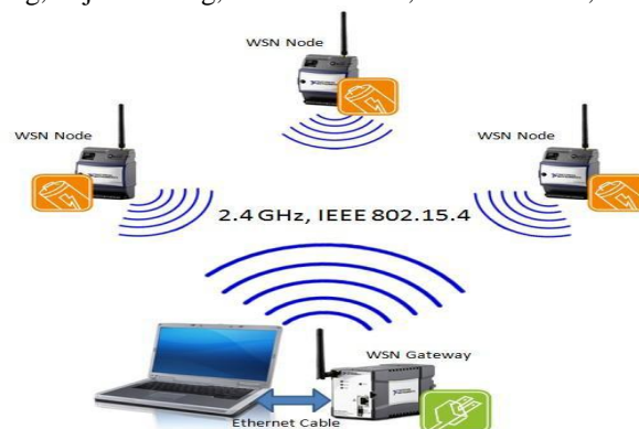
Fig .1: Communication between WSN nodes
