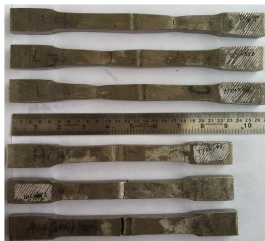
Figure 5: Fracture features of transverse tensile tested specimens showing the location of fracture.
