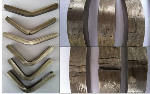
Figure 7: Fracture features of Bend tested specimens showing the location of fracture On Low and High Heat input Welded Joints.
