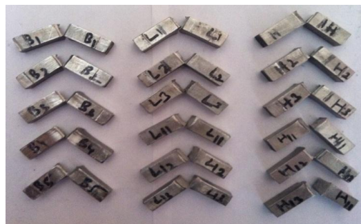
Figure 5: Fracture features of impact tested specimens showing the location of fracture.
