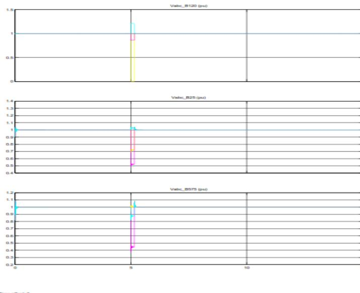
Fig. 13 Voltage at PCC for LG fault in UPFC compensated system with Resistive Load
