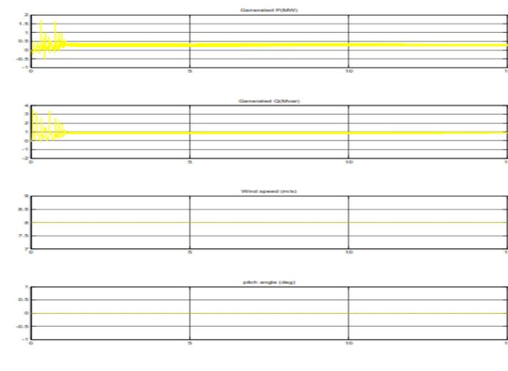
Fig. 7 Reactive power at PCC for LG fault with Resistive Load.
