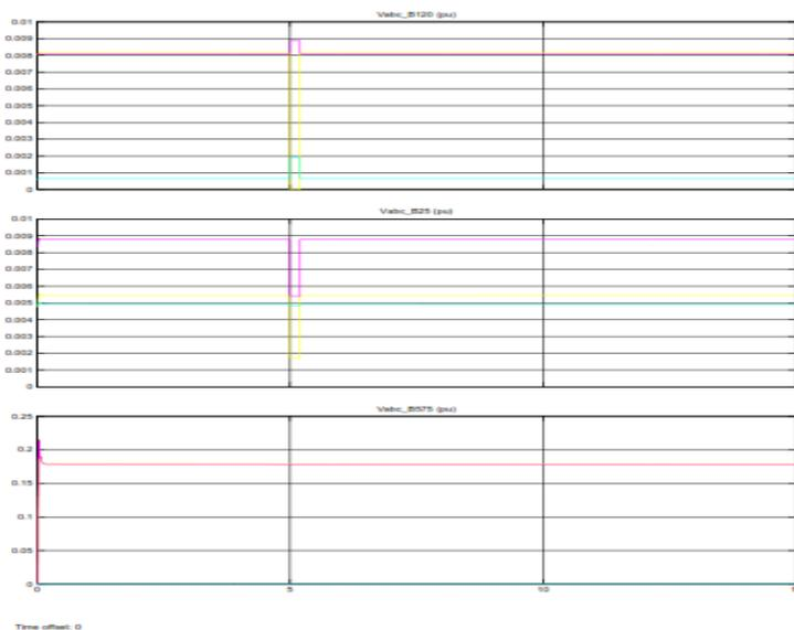
Fig. 6 Volatge at PCC for LG fault with Inductive Load.
