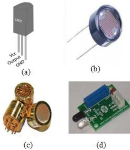
Fig.7. Sensor Nodes<sup>11</sup>: (a) Temperature Sensor (b) Light or LDR Sensor (c) Carbon-dioxide Sensor and (d) IR Sensor
