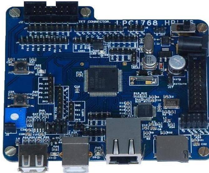
Fig.6. 32-Bit ARM Cortex Microcontroller Unit<sup>11</sup>
