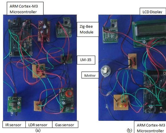
Fig.8. Developed monitoring system (a) Transmitter/ Input end (b) Receiver/Output end
