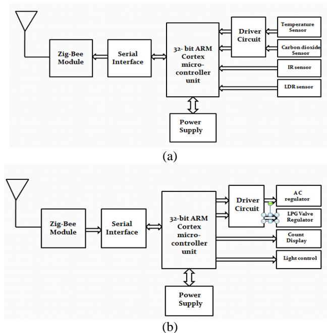
Fig.5. System Architecture: (a) Input/Transmitter End and (b) Output/Receiver End
