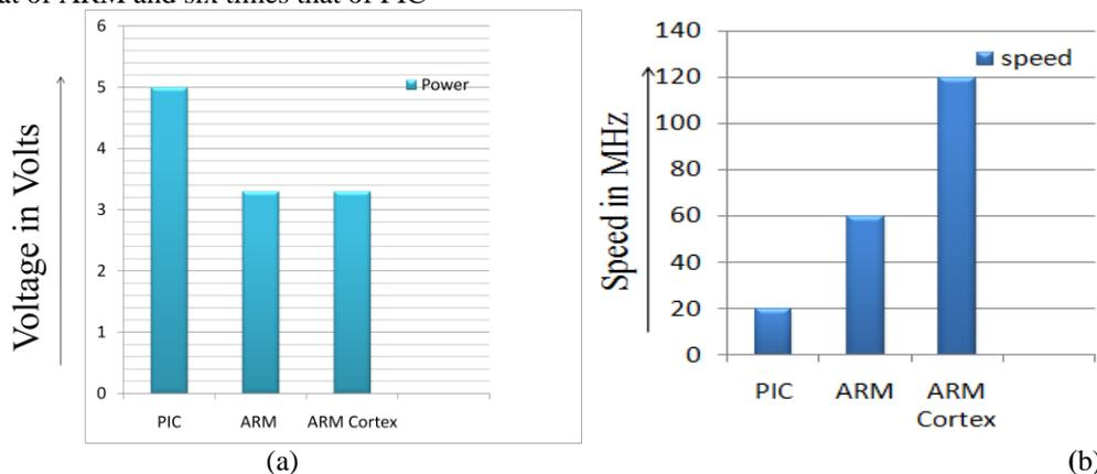
Fig.8.Comparison of PIC, ARM, ARM Cortex in terms of a) Power and (b) Speed
