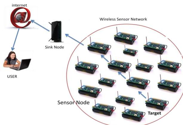
Fig.1. Typical multi-hop wireless sensor network architecture
