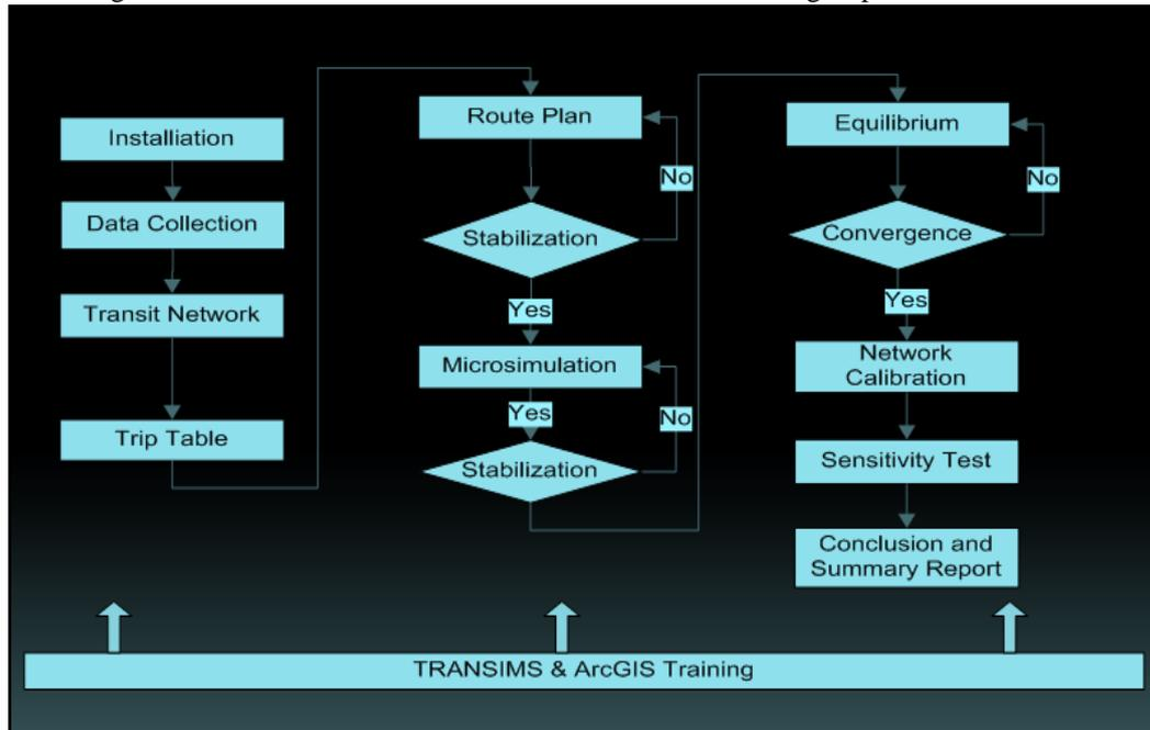
Figure. 2 TMC TRANSIMS Project process flow chart
