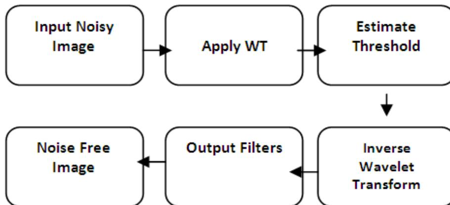
Figure 1.1: Image Noise Removal by WT
