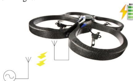
Fig.15 Example of drone charging through antennas in microwave power transmission.
