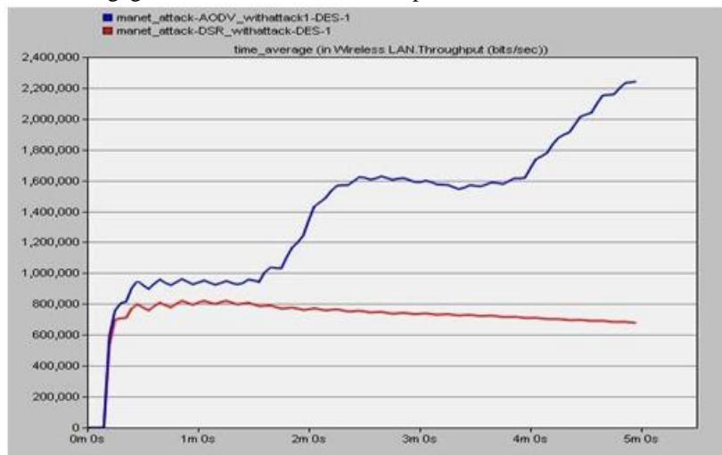
Figure14. Throughput of the network after attack under AODV and DSR protocol
