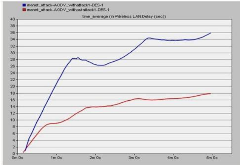
Figure9. Detection of physical jamming attack under AODV on the basis of delay
