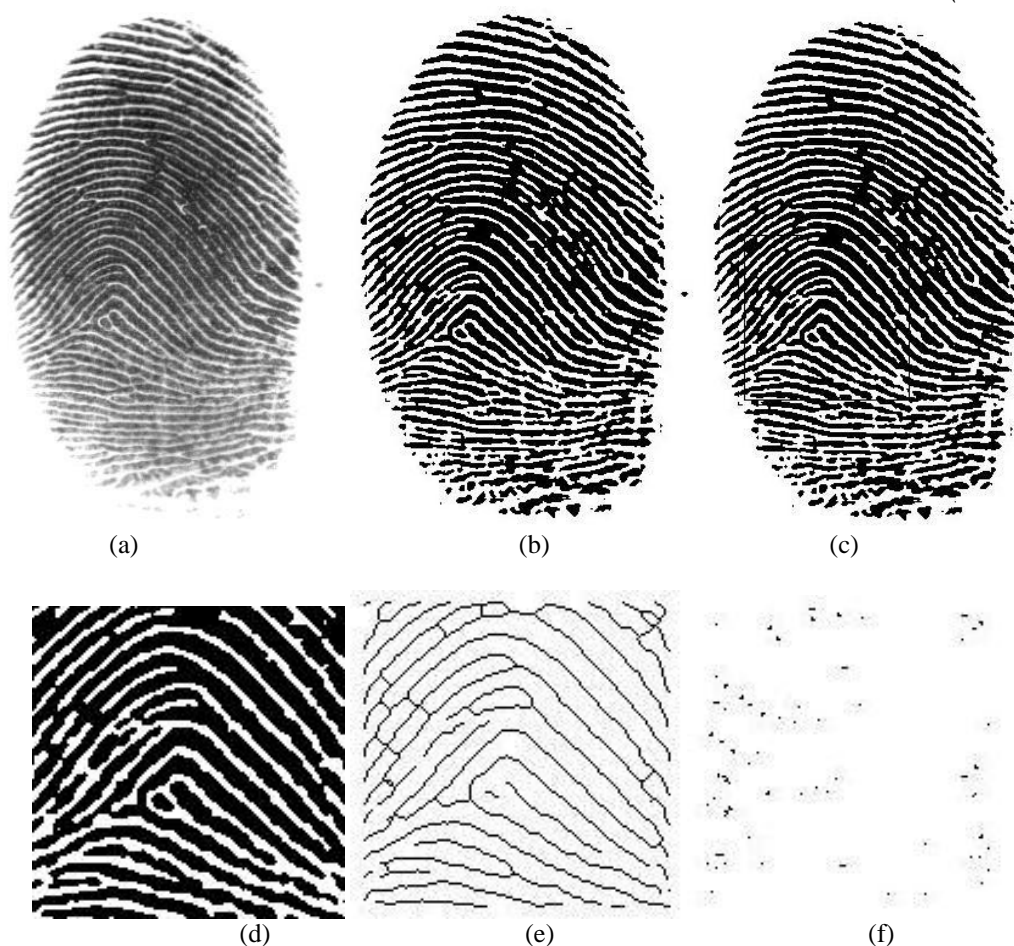
Figure 9: Result of pre-processing steps. (a) original image, (b) image after noise reduction and normalization, (c) region of interest, (d) cropped image, (e) thinned image, (f) extracted minutia.
