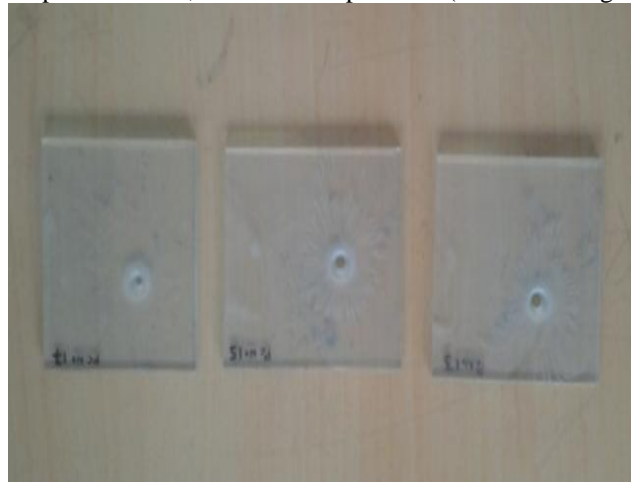
Figure 3: Machined Work Piece with variable Nozzle
