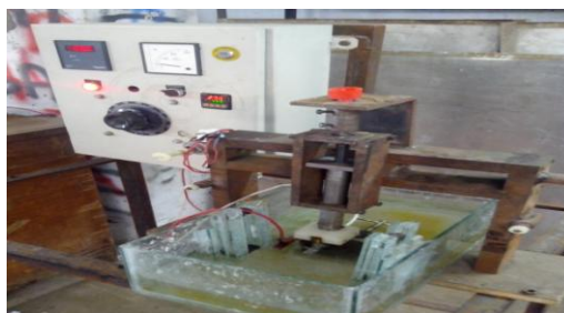
Fig. 1: Micro Machining of Aluminium Alloy at Micro ECM
