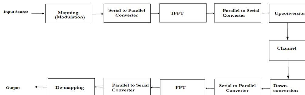
Fig. 1 Basic OFDM System block diagram
