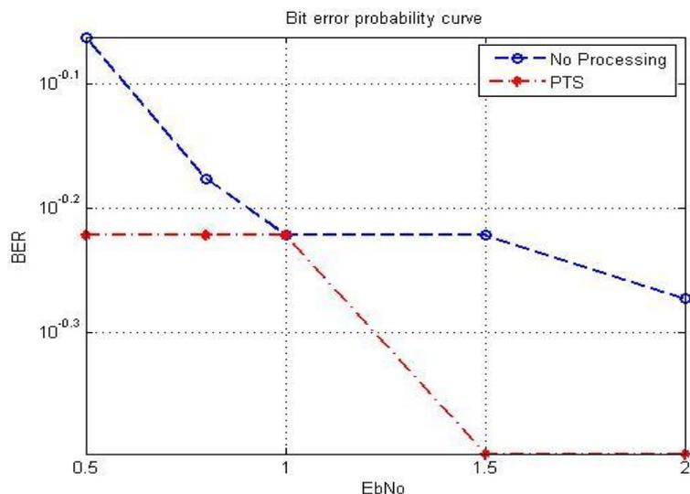
Fig. 5 BER Performance curve for proposed system (MATLAB Result)
