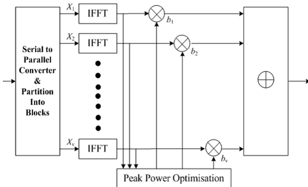
Fig. 2 The functional block diagram of partial transmit sequence based PAPR reduction algorithm
