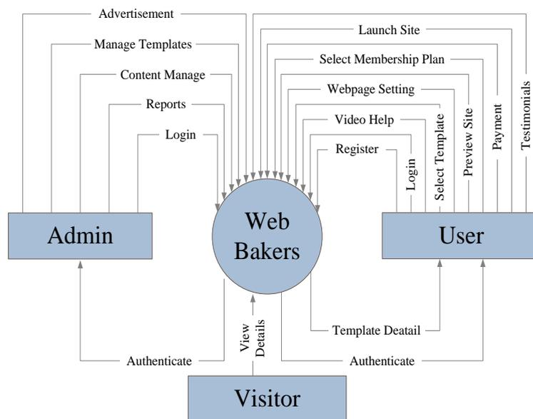
Figure: A Context level Data Flow Diagram
