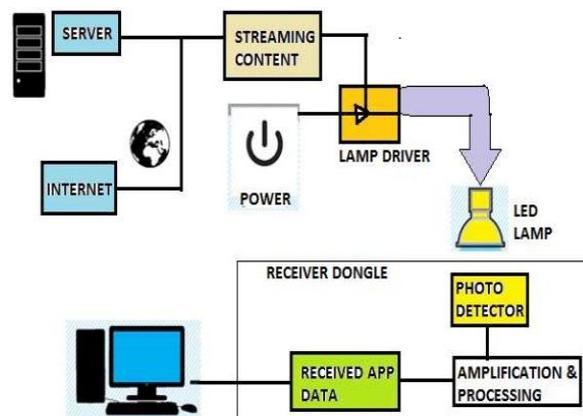
Fig. 4 Data transmission using LED
