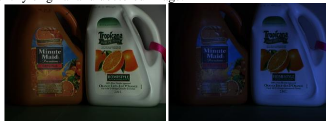
Fig. 2 Example of the influence of illumination on the perceived object color. The same scene is shown, once exposed to white illumination, once exposed to illuminants that approximate illumination at night.
