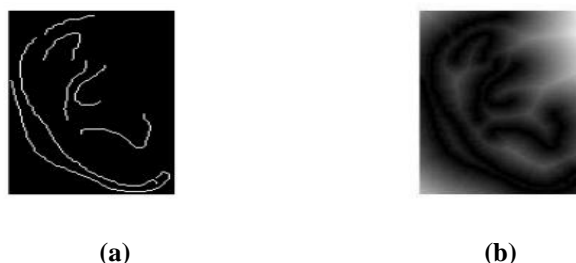
Fig. 2.3.(a) Edge map, (b) distance transform of (a) Zernike Moments:
