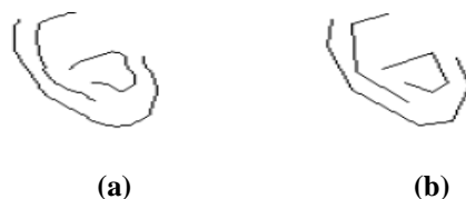
Fig. 2.2. (a) Original edge image, (b) Edge image after approximating edges with line segments
