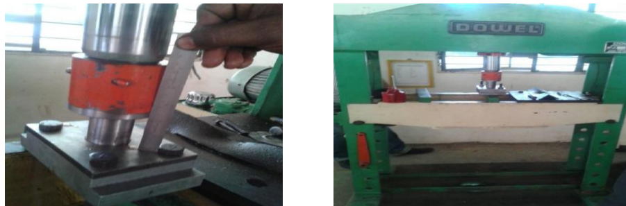
Fig 1.3 Experimental set up for performing Deep Drawing operations
