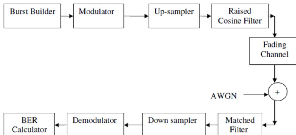
Figure 6 Physical Layer simulation of a wireless communication system
