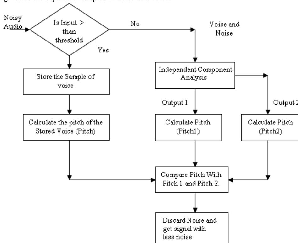
Figure 3 Initial block diagram of the ICA based call drop reduction system
